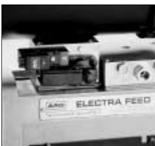
Solenoid kit part no. 49787 for remote control port.
